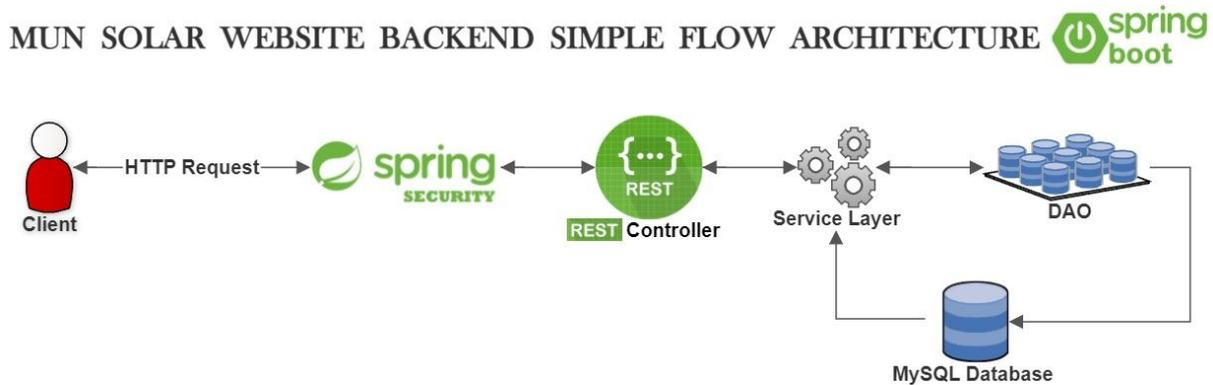
Fig. 6. Block diagram of the web-based monitoring system.
