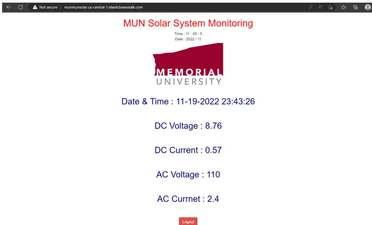
Fig. 11. Web-based SCADA real-time monitoring.
