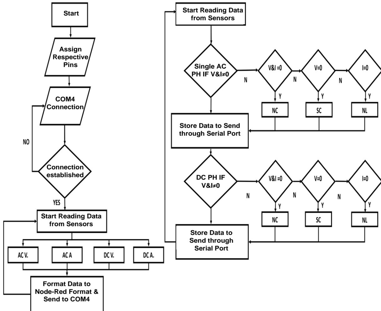
Fig. 4. Block diagram for the Arduino code.
