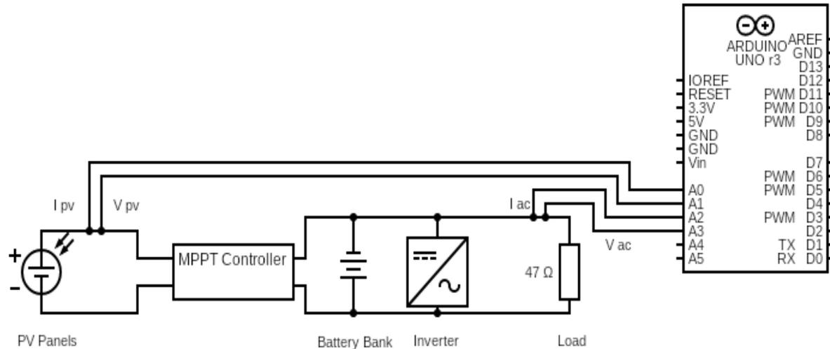
Fig. 2. Arduino connection layout.
