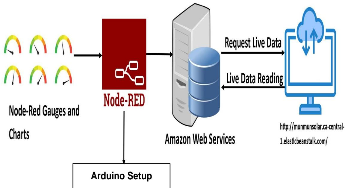
Fig. 1. Block diagram of the SCADA web system.
